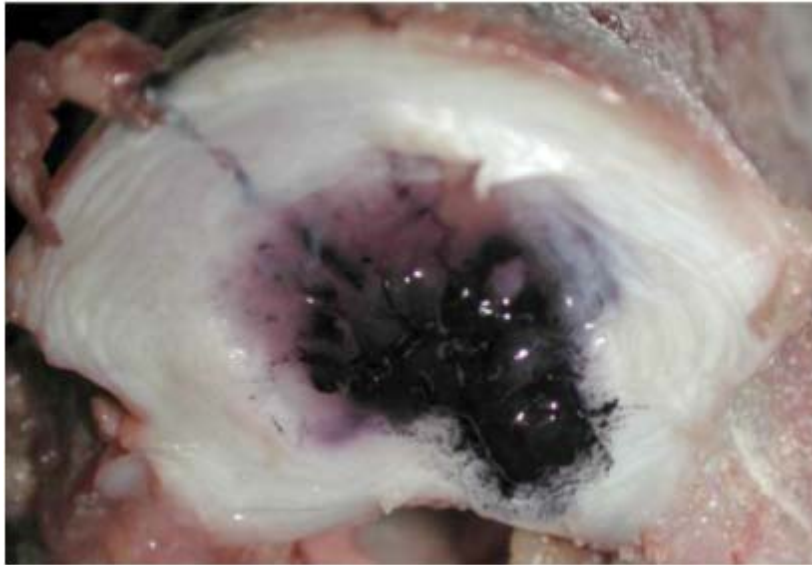
Figure 5. Photograph of a sectioned disc post fatigue load. After axial loading combine with left anterolateral flexion fatigue loading, the nucleus pulposus protruded toward the right posterolateral side of the disc.
